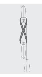
Breakaway safety tassel is pre-fitted to the lift cords so that when a horizontal force is applied to the cords entering the condenser it safely breaks away eliminating any hazardous loops.
